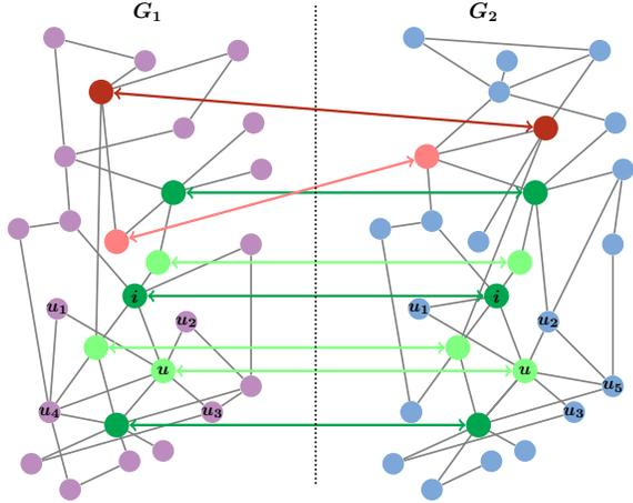
**Figure 1: NoisySeeds Algorithm: Dark green and dark red nodes correspond to the initial correct and wrong seed pairs, respectively. After the first four iterations (for  $r = 2$ ), light green nodes form correctly matched pairs, and light red nodes form wrongly matched pair (see Example 1).**
