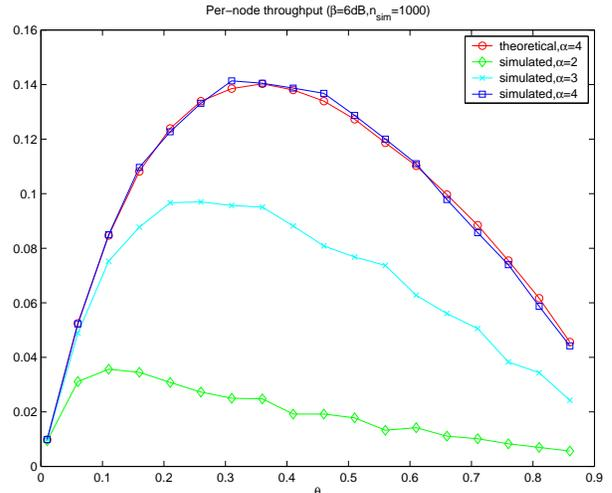
Figure 4: The normalized per-node throughput, as a function of the sender density  $\theta$ , for different values of  $\alpha$ . For  $\alpha = 4$ , the throughput predicted by the model is also shown.
