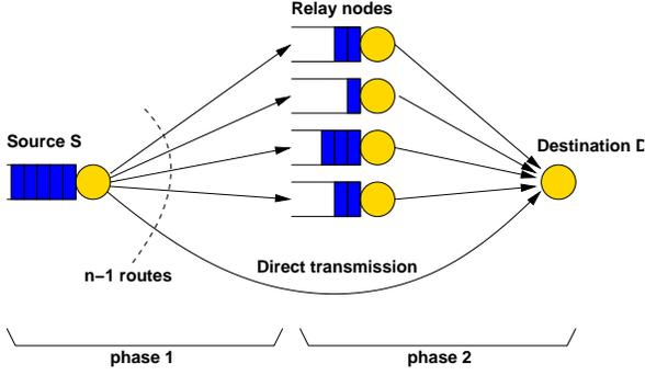
Figure 1: The two-phase scheduling policy viewed as a queuing system, for a source-destination pair: in phase 1, a packet at  $S$  is served by a queue of capacity  $O(1)$ , and is forwarded either to the destination or to one of  $n - 2$  relay nodes with equal probability. The service rate at each relay node  $R$  is  $O(1/n)$ , for a total session rate of  $O(1)$ .
