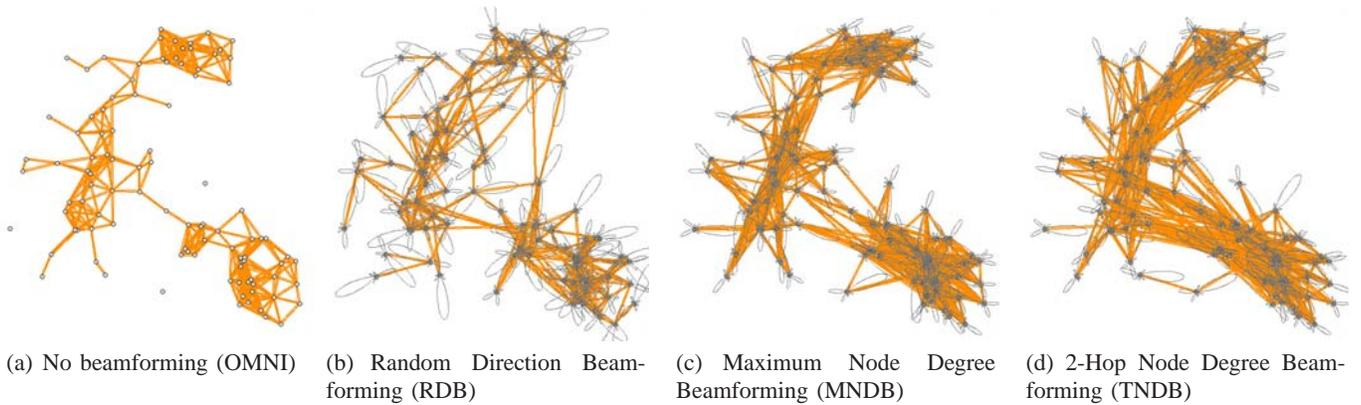
Fig. 1. Sample topologies resulting from the different beamforming approaches, for  $n = 100$  nodes with inhomogeneous (clustered) node distribution. In general, beamforming provides better connectivity than omni-directional antennas. Further information about the neighborhood can be used to significantly improve the resulting topology as evidenced for MNDB (one-hop information) and TNDB (two-hop information).
