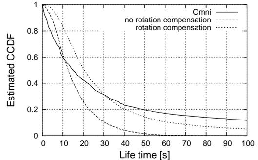
Fig. 8. Route life time with random direction mobility model for 100 nodes on  $1000 \times 1000 \text{ m}^2$ .
