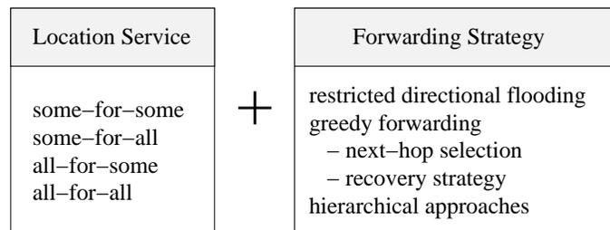
Fig. 1. Building blocks and criteria for classification
