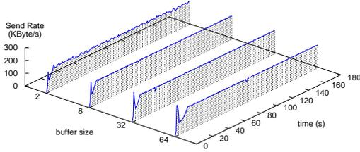
Figure 4: TFRC flow over Dummynet: oscillations prevented
