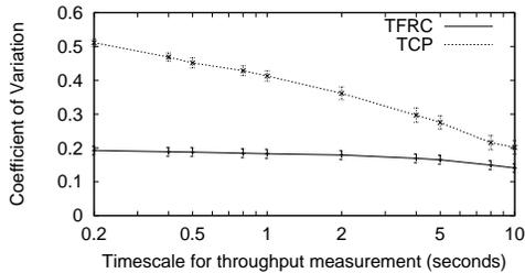
Figure 10: Coefficient of Variation of TCP and TFRC
